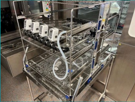
Loading rack with 2 levels for standard and special instruments (Robotic MD, DaVinci)
